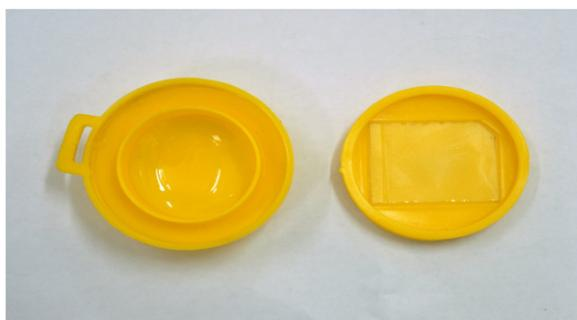
**Figure 1.** A photograph of the NRPB dosimeter.
